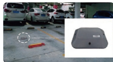
Smart Parking (Geomagnetic)
